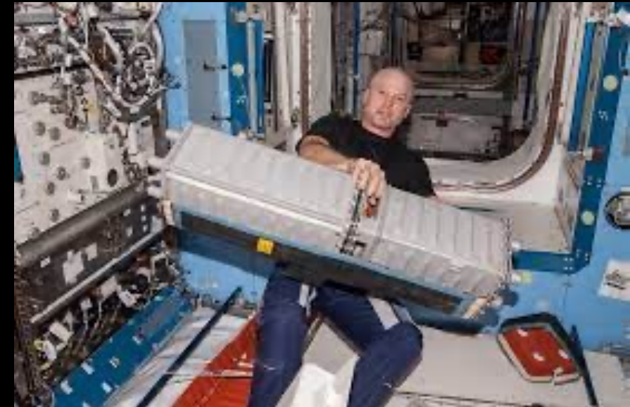
Carbon Dioxide Removal Assembly
